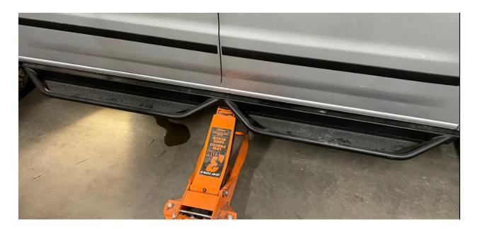
2. Use a permanent marker to mark the body of the van where the mounting bracket holes line up. Mark the hole in the lower mounting bracket flange, as well as the lower hole in the upper flange. The upper hole in the upper flange is there as a backup and does not need to be marked and drilled unless there are issues with the lower hole alignment.
