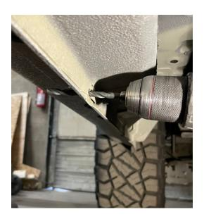
4. Use a hole starter punch or screw to put pilot holes in the upper hole marks to make it easier to drill at an angle. Drill holes to 5/16".
