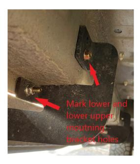
3. Remove the side step from under the van. Drill the lower flange holes through to a 1/4".
