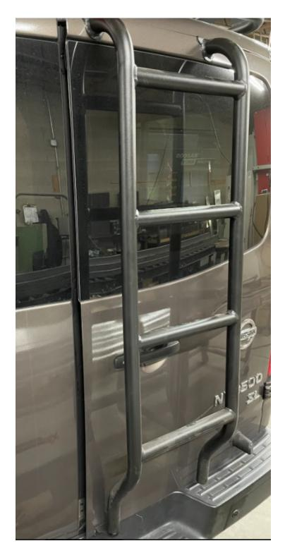
6. Install the two lower ladder brackets onto the lower edge of the van door and secure to the ladder using the included bolts and a 9/16" socket.
