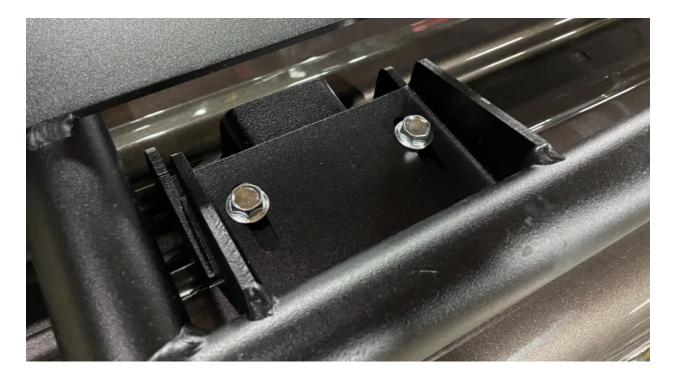
4. Make sure protective adhesive material is applied to the mounting pads of the ladder and ladder brackets. This should be applied before the ladder is shipped to you.
